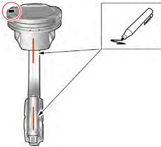
**Caution! Note the position of the component before removal.**
