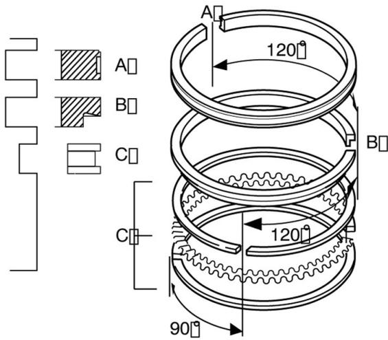
**Caution!** Make sure that the piston rings can be easily rotated by hand in the piston ring grooves.
