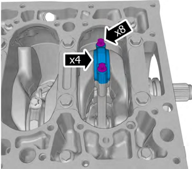
**Warning!** Make sure that new bolts are installed.
